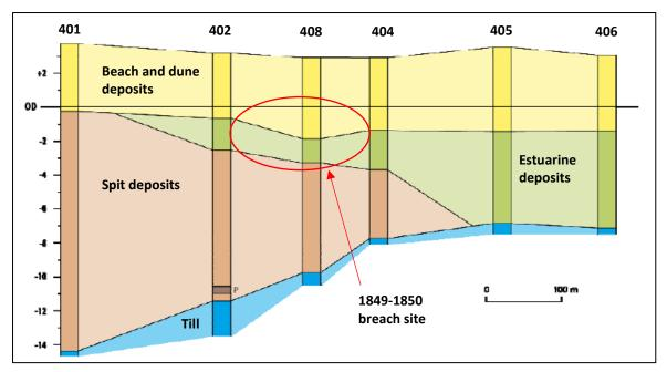
Figure 31 BGS borehole investigation at the 1849/1850 breach site (from Balson 2008).
